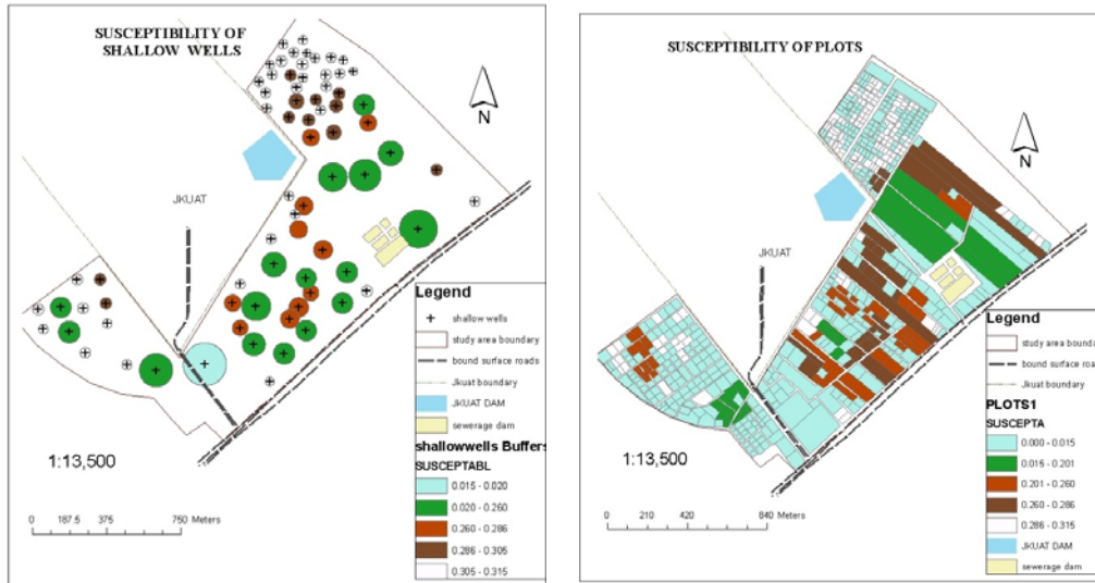
Figure 6: Map showing susceptibility levels for the buffered shallow wells; Figure 7: Map showing susceptibility levels of each plot
