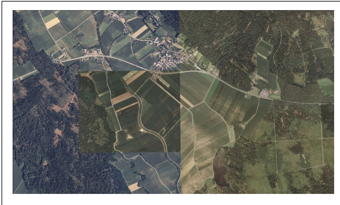
Figure 1: Screenshot of Virtual Earth - sample for problems with image data fusion, especially problems arise in homogenous regions (source: http://maps.live.com , accessed on 2009/04/30)
