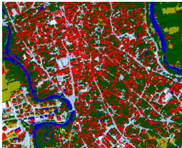
Figure 6: Results of Object-Based Classification of Ikonos Image in Bartın city center
