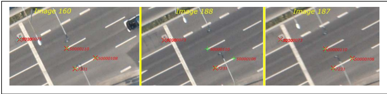
Figure 8: Sample of automatically extracted tie points
